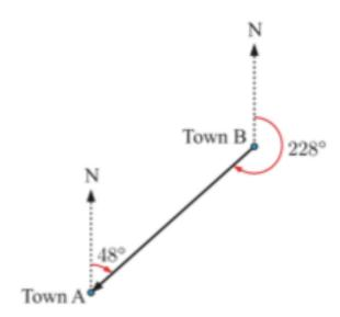
The bearing of B from A is 048°. The bearing of A from B is 228°.
